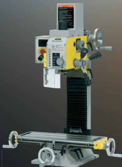
**BOHR - FRÄSMASCHINE BFM 20 Vario**
