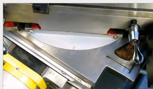
cross table rotation 45° to the left and right
