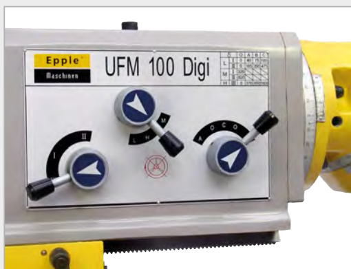
control panel for 11 spindle speeds
