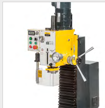
Open control unit with thread cutting device
