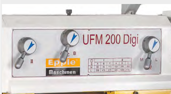
control panel for 12 spindle speeds
