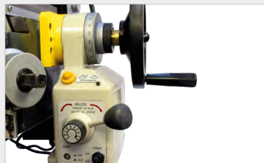
Y-axis with stepless feed control
