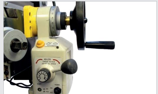
Y-axis with stepless feed control
