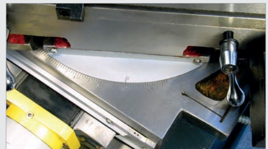
cross table rotation 45° to the left and right
