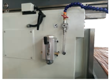
PIC: central lubrication
