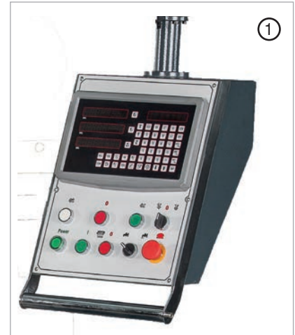
DIGI model with easy to operate LED display for precise position readout and measurement of traverse.
