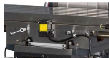
Precision grinding hardened table swivel from -45° to +45°
