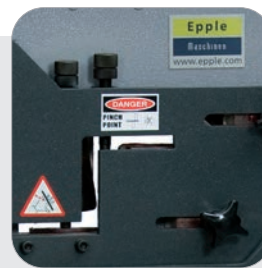
angle iron station 45/ 90° angle
