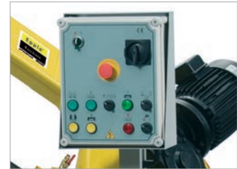
Rotatable and ergonomic designed control panel
