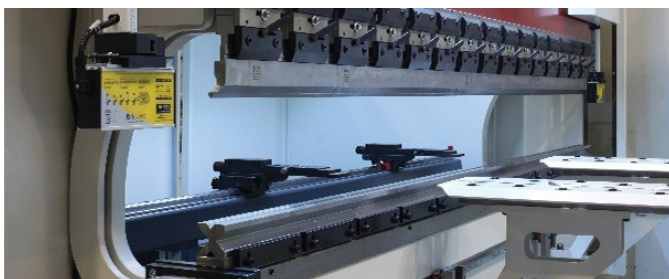
PIC: WORKING AREA PRESS BRAKES (E-GBP 2.550-120 CNC) WITH SPECIAL ACCESSORIES QUICK-CHANGE HOLDERS AND SHEET LIFTING HOLDER
