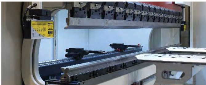
PIC.: WORKING AREA PRESS BRAKES (E-GBP 2.550-120) WITH SPECIAL ACCESSORIES QUICK-CHANGE HOLDERS AND SHEET LIFTING HOLDER
