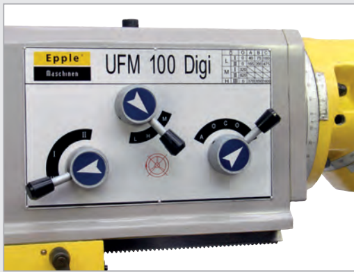
control panel for 11 spindle speeds
