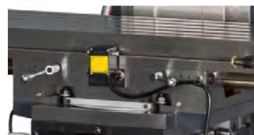
Precision grinding hardened table swivel from -45° to +45°
