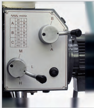
X- and Y-axes with 9 table speeds
