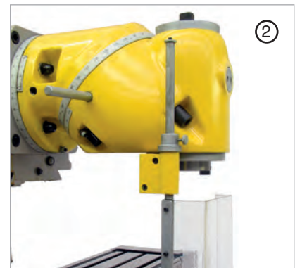
DIGI model with easy to operate LED display for precise position readout and measurement of travel distances. DIGI-Machines exclusive.
