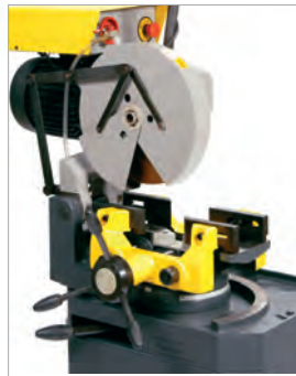
PIC.: head for slitting 90° pivoted
