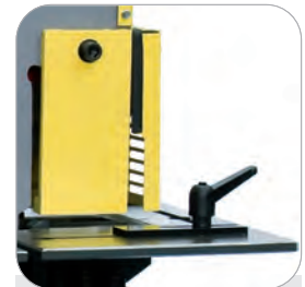
notching station Table with arrester and scales
