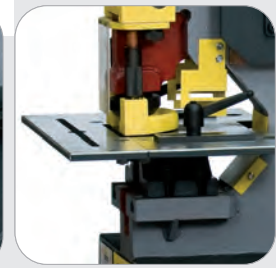
punch station Max. capacity 28 x 15 mm and 38 x 11mm
