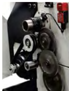
Frequency motor drive Fast shifting gears
