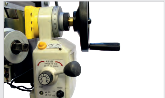
Y-axis with stepless feed control
