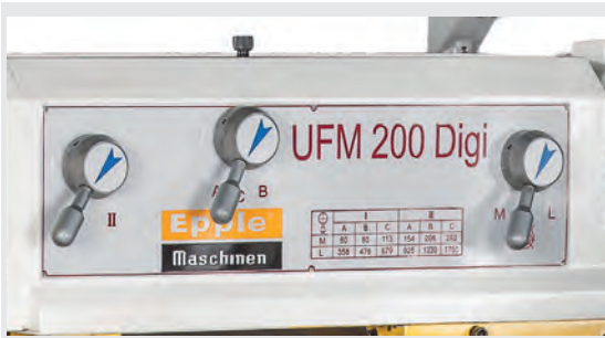
control panel for 12 spindle speeds
