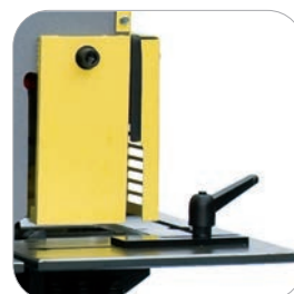
notching station Table with arrester and scales
