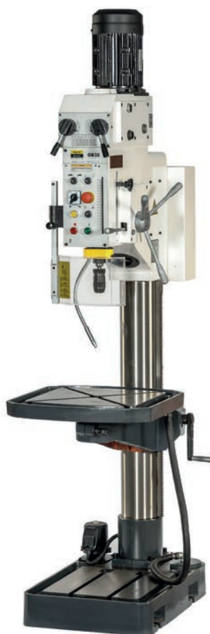
PIC: GB 32 automatical mechanical feed
