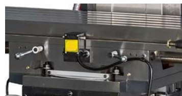
Precision grinding hardened table swivel from -45° to +45°
