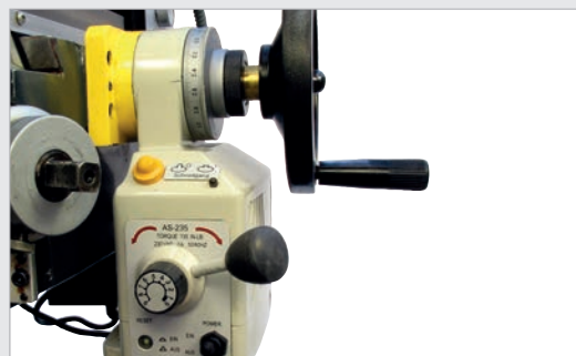
Y-axis with stepless feed control
