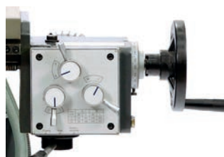
Automatic feed for the X-axis as standard (8 speeds)
