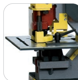
punch station max. capacity 28 x 15 mm and 38 x 11mm
