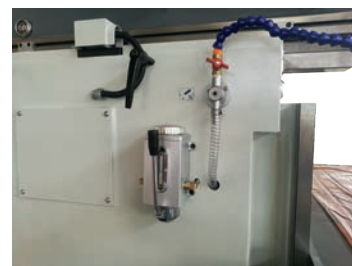
PIC: central lubrication
